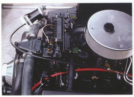
This photo shows a good installation of servo-motor and cable (smooth bend in cable).
