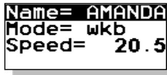
Scroll through the alphabet using **UP & DOWN** keys, and then press **MENU** to move to next position. Press the **MENU** key to move through the settings. If you are programming a JUMP or SLALOM name there will be another page of settings to enter.
