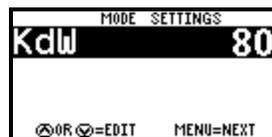
**KDW (Throttle Pull Rate)** – KDW can be changed using up or down keys. The higher the value, the more aggressive the control. Heavy boats may need higher values. Factory setting is about 80. Normal range is 40 – 120. (If this value is set too high, the control may become a little erratic and engagement may not be as smooth).
