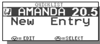
**Creating Names** – First enter the Quick List. Press the **MENU** key until [NEW ENTRY] is highlighted. Then press the **UP** key to enter a new name. The following screen will then appear:
