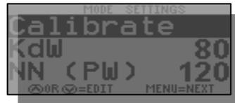
**KDW (Throttle Pull Rate)** – KDW can be changed using up or down keys. The higher the value, the more aggressive the control. Heavy boats may need higher values. Factory setting is about 80. Normal range is 80 – 200.
