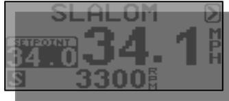
This mode allows you to set speeds in 2 mph increments ranging from 24 – 36 mph. It is designed for those wishing to use the system for open water skiing.
