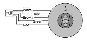
Red – 12-V Power Bare – Ground Green – Speed White – Water Temp Brown – Water Temp
