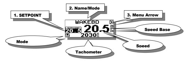
2. RPM Mode where the user sets an rpm value. Designed for higher speed use such as open water skiing or cruising.
