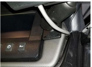
Photo shows alternative mounting location and wire routing.
