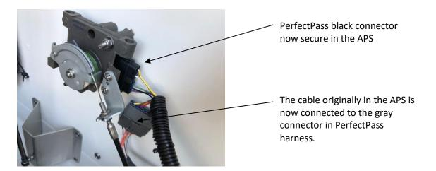
The seven foot harness will be routed carefully across to the Port side where you will repeat this process on twin engine boats.
