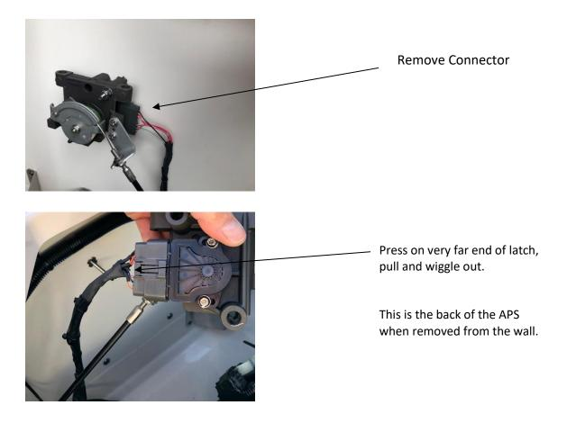
NOTE: These connectors can be unusually tight so removing the APS from the side wall (2 nuts) using a 7/16 nut driver gives much easier access to removing the connector.
