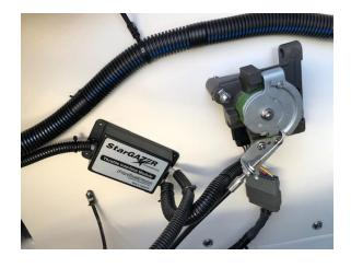
Shows Throttle Interface Module mounted to starboard side wall and cables connected.
