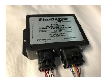
Shows Master Module after both engine control harness and display gauge are connected.
